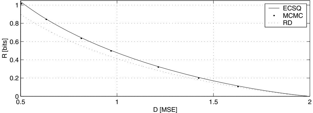
Figure 1. Comparison of entropy coding (ECSQ), Algorithm 1 (MCMC), and the RD function. ( $n = 10^5$ ,  $|\mathcal{Z}| \in \{3, 5, 7\}$ ,  $r = 100$ ,  $k \approx \frac{1}{2} \log_{|\mathcal{Z}|}(n)$ , and  $c = 1.6$ .)
